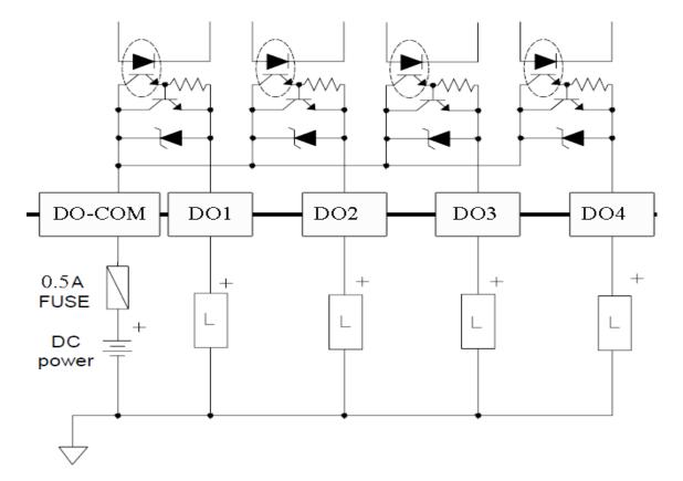
• Note that the above output is a SOURCE digital output (that is, it can only connect and disconnect the positive voltage).
